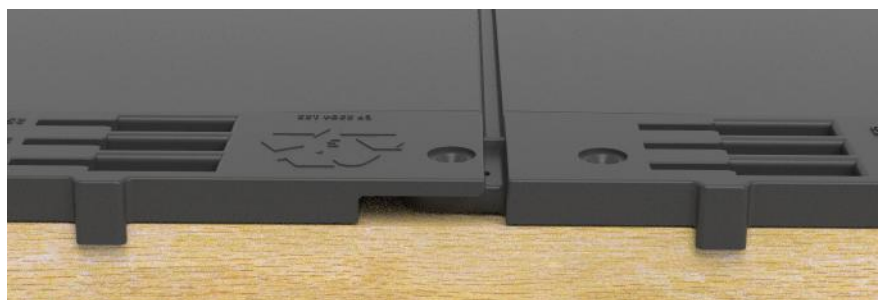
Each tile has two detachable nibs (F) at the top. These are used to hook the tile over the batten. When a batten has been fitted out of alignment or there has been some movement after fitting, the installer can break the nibs off as required if they find that the nibs no longer hook over the batten.
